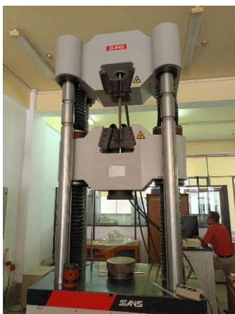
Figure 8: Tensile testing using universal test machine in the laboratory
