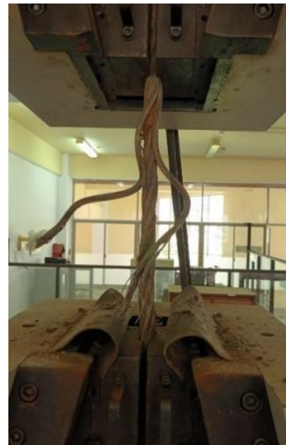
Figure 9: A view of the broken wire rope
