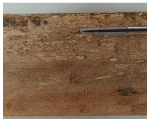
Figure 11: Hora timber sample and bottom cracks after bending test
