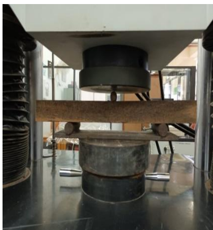
Figure 10: Bending test on Hora timber sample
