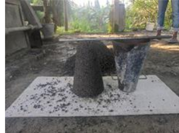
Figure 5: Slump cone test
