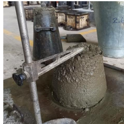
Figure 4: Slump of 95 mm for conventional concrete
