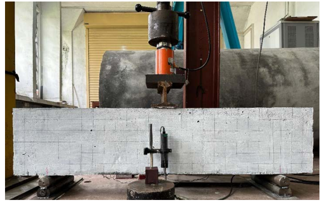
Figure 7: Test Setup for Beam Tests
