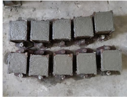
Figure 3: Concrete cubes just after casting
