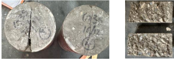
Figure 12: Failure plane of BST specimens
