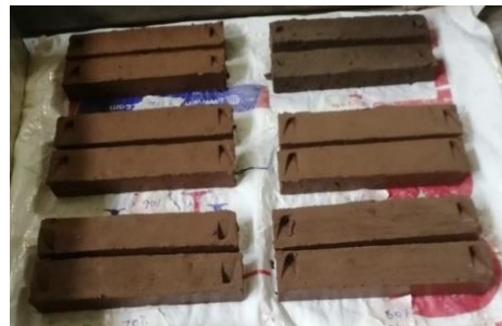
Figure 6: Samples for check dry shrinkage and firing shrinkage
