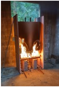
Figure 6: Flame Spread during the test
