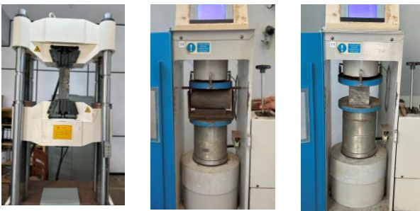
a) MDTT done using the Universal Testing Machine b) BST and CCT done using the Compression Testing Machine
