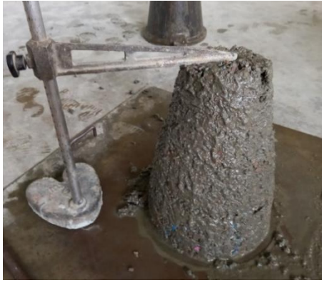
Figure 5: Slump of 40 mm for PP100%-FA20% concrete
