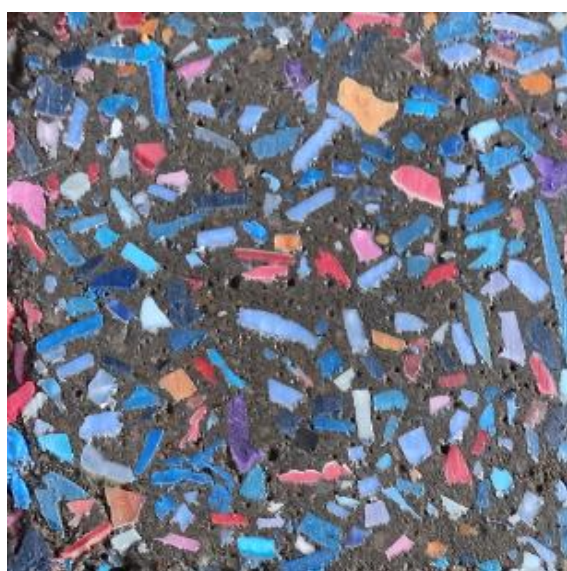
Figure 8: Cut surface of PP-modified concrete cube specimen (not to scale)
