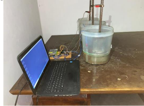
Figure 1: Accelerated corrosion setup and testing
