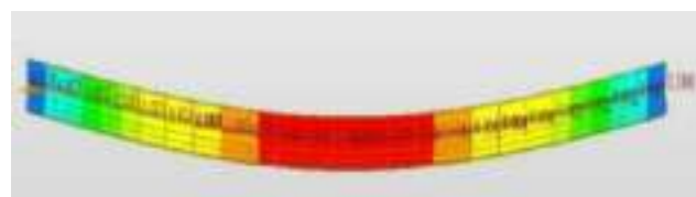
Figure 8: Deflection due to self-weight of the girder
