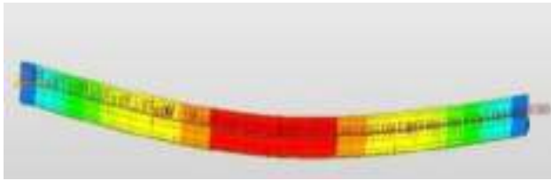
Figure 10: Deflection due the point load
