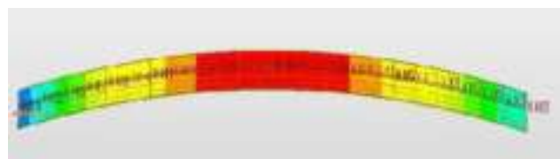
Figure 9: Deflection due to prestress force
